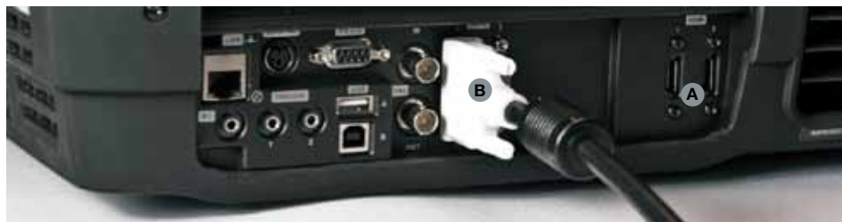
Figure 1-5. Connecting a computer source
